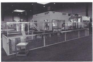
MMS 500 with tool changing magazine, circular table, pallet transport trolley and pallet storage locations ... with and without casing.
